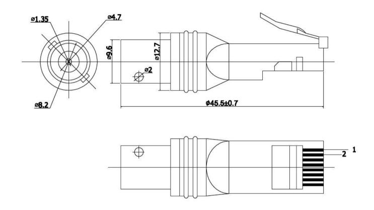
1: Connecting ---- BNC Conductor; 2: Connecting ---- BNC Grounding
