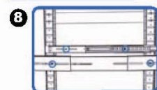
8 Repeat previous steps to secure sliding rails on both sides.
